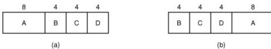
Figure 2-24. An example of shortest job first scheduling. (a) Running four jobs in the original order. (b) Running them in shortest job first order.
